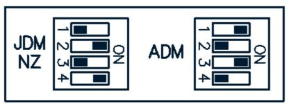
If your ECU bottom board is version 1.2 or higher, you will have a second set of jumpers. The jumpers are used to configure the board for either a 1991 - 1993 or a 1994 - 2002 SR20DET.
