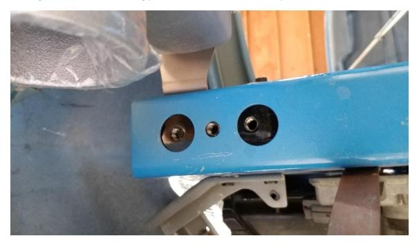
3. The tow hook can be arranged one of two ways on either side. To have the tow hook come out through the main duct, arrange the spacer so that it is between the tow hook and the box frame.
