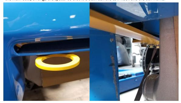
4. To have the tow hook come out through the slot vent, mount the tow hook directly against the box frame.
