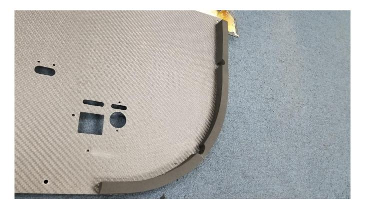
8. Install the provided offset spacers. The hole nearest the speaker can be reached by removing the speaker. Reinstall the speaker after installing the spacer. Leave the bottom forward most screw out. This will be replaced later in the install. Before installing the new door panel assembly, the door should be cleaned of any glue and deadening that may show. The OE Plastic shrouding may be removed or taped back for a cleaner install.
