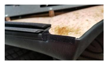
6. Mount the new door panels to the original upper sections. Reuse the existing hardware from the original panel. Note that there is a different set of mounting holes for AP1 and AP2 door panels. The rear most mounting hole is not used on AP2.
