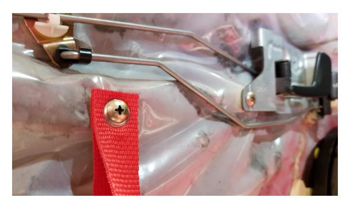
10. Slide the top panel section into the door first. Lift the bottom of the panel outward slightly and plug in the mirror and window controls.
