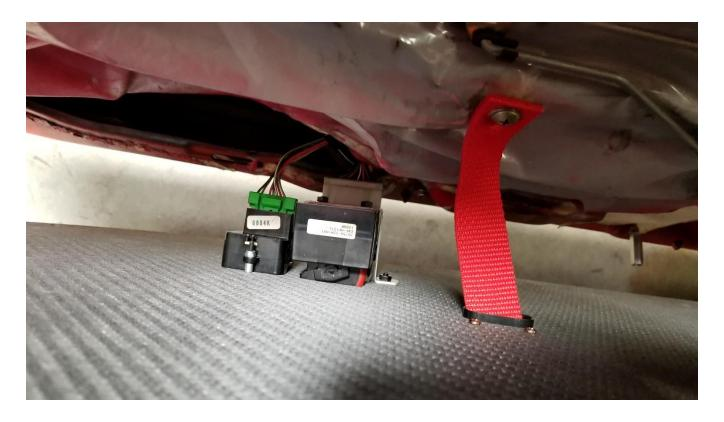
11. Use the #10 tapping screw and 25mm #10 spacer for the mounting hole closest to the speaker. The bottom forward most speaker mount is used. Use the 20mm M5 screws and 10mm spacer for the next mounting point back. Fasten the remaining mounting holes using the 10mm M5 screws.
