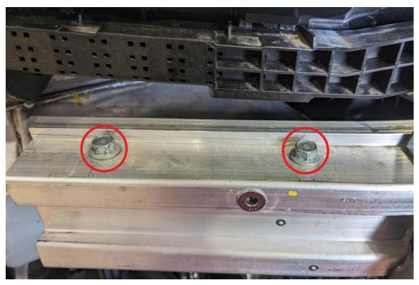
6. Slide the EVS Tuning Tow adapter over the crash beam and fasten using the included 120mm long M10 bolts. Torque to 32 ft-lbs. Then install the M10 lock nuts and washers over the protruding end at the bottom.
