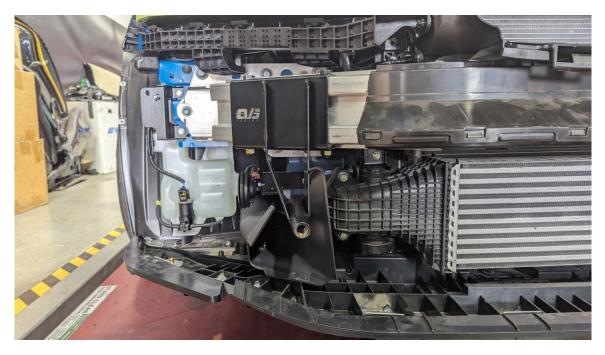
7. Reinstall the upper air guide and brake duct.
