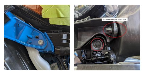
3. Remove the passenger(right) side brake duct and trim using the included templates:
