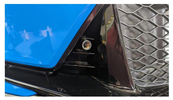
10. Install the EVS Tuning folding tow ring. The locking nut is 24mm wide.
