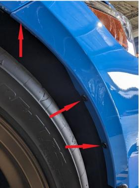
2. Remove the passenger(right) side headlight. The following photos highlight screws and clips holding the headlight in.
