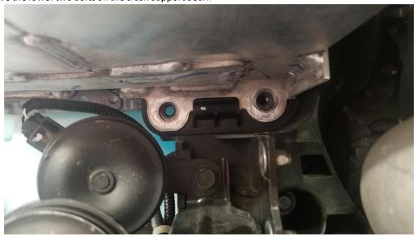
4. Mount the Tow Hook Adapter using the supplied 50mm bolts as shown below.
