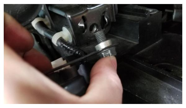
3. Remove the lower two bolts on the crash support beam
