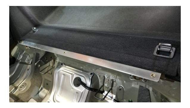
5. Carefully align the rear seat delete panel over the mounting bracket and attach using the supplied M6 button head screws. Start with the forward screws in the center and work towards the back.
