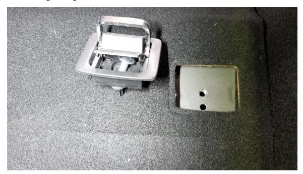
4. Align the rear mounting bracket as pictured below and reinstall the OE cargo rings over the bracket.
