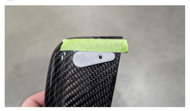
4. Install the provided dowel pin in the hole near the stem base.
