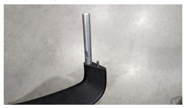
5. Reassemble the mirror housing with the hole aligned to the pin at the stem base.
