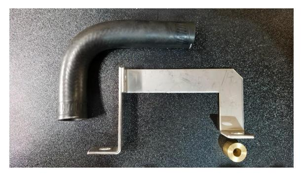
3. Install the factory bracket on the SSQV pipe using the factory bolt.
