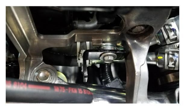
6. Install SSQV Assy using HKS Bolt M8-15, spring washer and flat washer as in the photo below.
