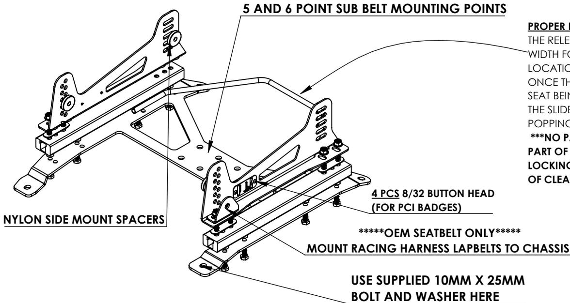
**PROPER RELEASE HANDLE INSTALLATION :**
