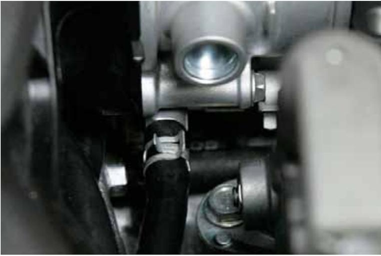
44. With the intake still off, now is a good time to hook up the water lines for the turbo. The shorter water line provided will hook up to this water line off the throttlebody, on the side and towards the back.
