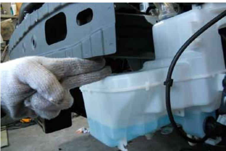
23. With those changes, the silicone pipe should fit in between the bumper beam and the water tank smoothly, and go up into the engine bay.
