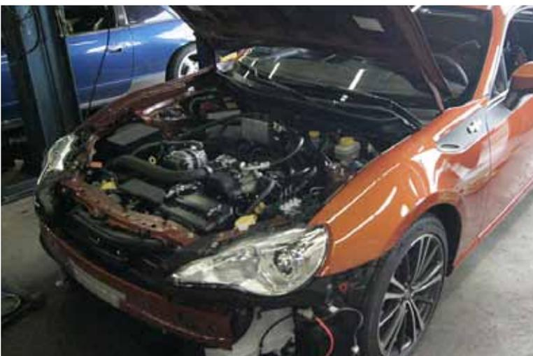
63. Fit the air box to the silicone inlet pipe, and fit the air filter back in place. Clamp the air box back up and fit the wiring harness to the MAF sensor. Check all your fittings, hoses, and other pieces, and make sure you've tightened up the exhaust. Now is a good time to do a test start of the car and make sure there are no leaks. If everything checks out, replace the bumper onto the car in a reverse process of the removal.
