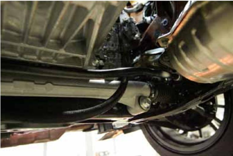
33. You can fit up the oil line to the oil pump at this time, and run it down towards the steering rack. It will be tucked up between the steering rack and the frame there, and run to the other side of the engine. Mount it up to the other hose running underneath the engine on that side, then leave it alone for now till the turbo is mounted up.
