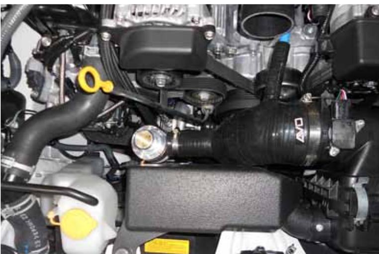
55. Now fit the air inlet pipe that will go from the airbox to the turbo. Fit it to the turbo first, and make sure it's clamped on tight. Run the breather line to the smaller fitting off the side, and clamp that in. Then prepare a clamp on the bigger fitting, this is where the BOV will fit into.
