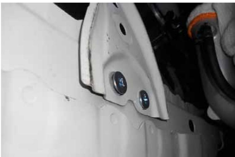
43. With it out of the car, you will need to modify it slightly at the bottom. As there will be silicone hosing resting against it once everything is installed, we recommend flattening down the outer edges so they don't cut into the silicone pipes. Then bolt it back in with the supplied rounded head bolts used at the bottom.
