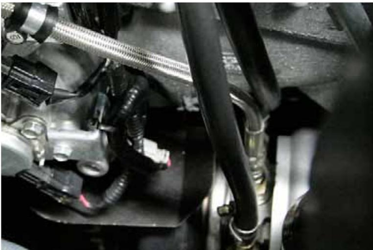
54. Fit the water lines to the turbo charger, one to each side on the supplied turbo water fittings. Clamp them down. Use supplied fasteners to keep the lines together, and away from the pulleys.
