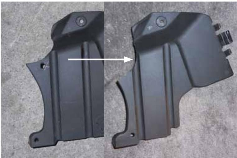
18. Fit the radiator air deflectors to the side to see where the silicone intercooler hoses will go, then trim them so that the hoses will pass through smoothly. Don't just discard these deflectors, they do an important job of keeping air going through the radiator!
