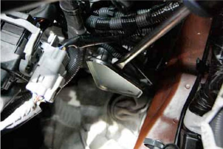
29. On that same side of the engine, look for this plate at the back of the head. Unbolt it, and then you'll need to lever it off as it's basically just sealed on with some silicone gasket sealant.
