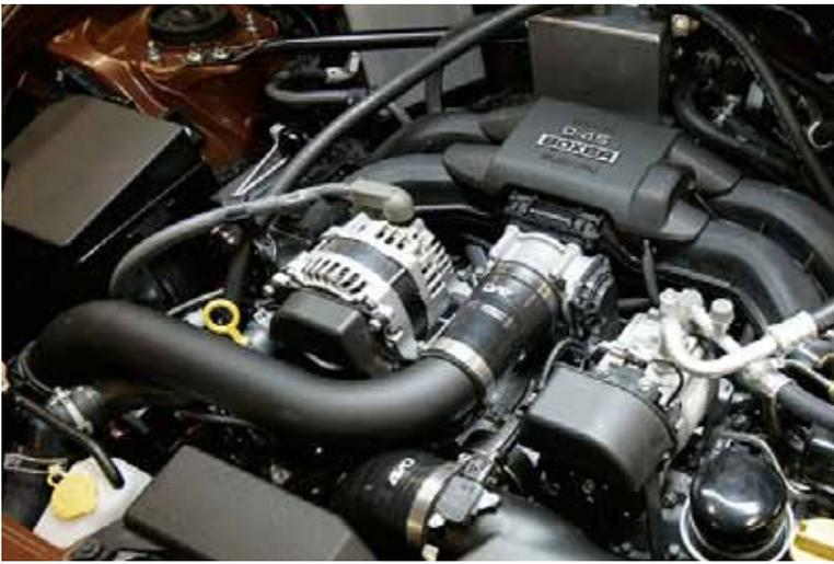
60. Fit the intake pipe to the throttle body, and clamp down the silicone hoses.
