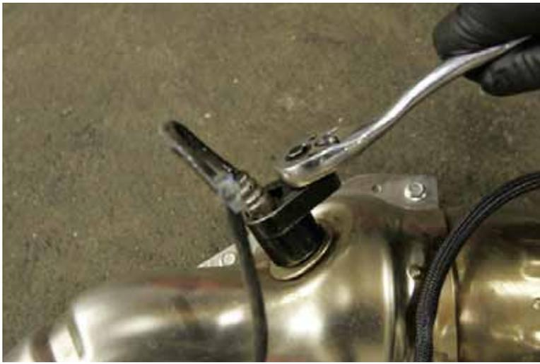
40. With the exhaust manifold fully off, remove the two oxygen sensors.
