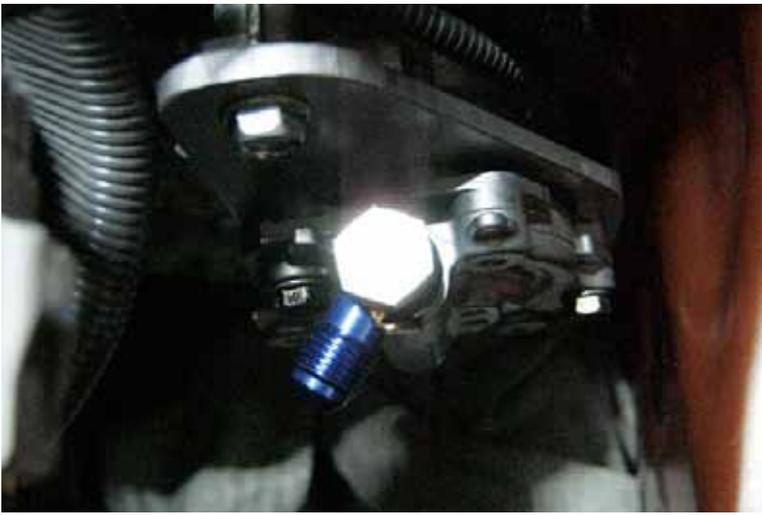
32. Now fully bolt the oil pump down to the plate itself - this process was to make sure the oil pump was situated properly. Fit it once more to the head to make sure it all lines up, if it doesn't, loosen the oil pump bolts off lightly and adjust. Once it's correctly set, put silicone sealant on the larger plate where it meets the head, and bolt the entire assembly in place.
