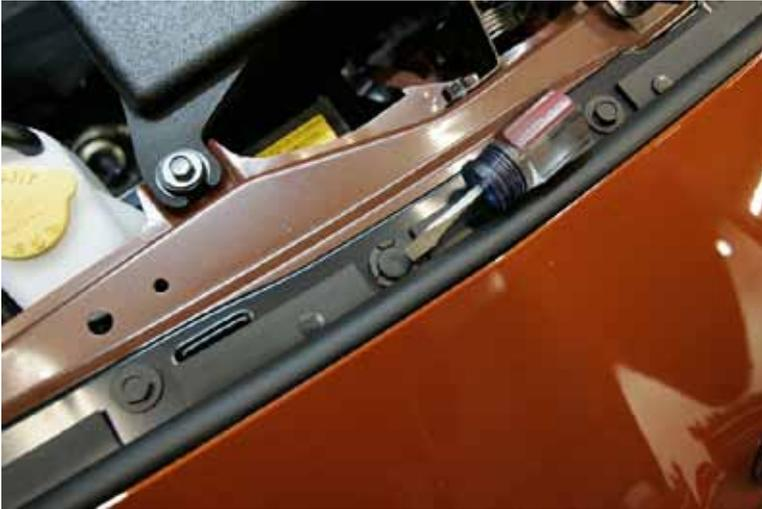
1. At the top of the bumper there is a several pop-its holding on a flat sectional piece. Remove the pop-it's with a screwdriver, then pull that piece up and off.
