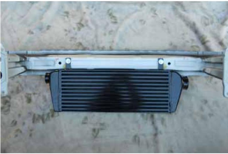
16. Screw the FMIC down to the bumper beam. Make sure it is snug against the bottom of the inner bumper beam.
