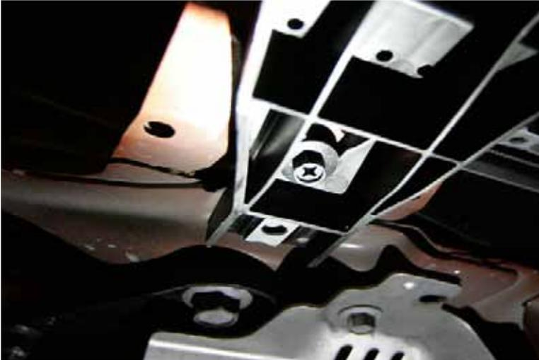
9. Underneath there is a series of bolts holding it on. Unbolt those with a socket wrench. With all these off, the undertray should come off smoothly. Put it aside for now.
