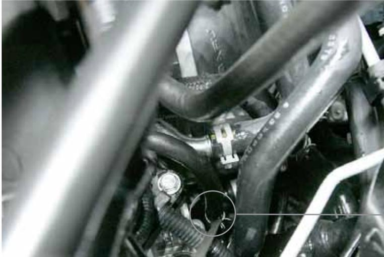
45. The standard water line reaches to the back of the engine here. Fit the longer water line here, after routing it underneath the intake manifold.
