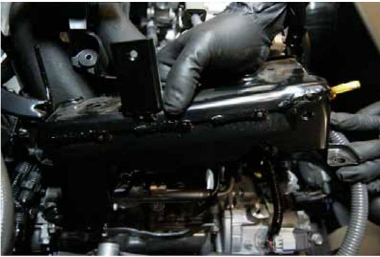
28. Once the wiring harness is unclipped fully, you will notice there is a small clip on it holding it to the black frame. Slide a screwdriver down and unclip it. Then with a socket wrench, remove the 3 bolts holding the black frame on (the one at the back is the hardest to get to), and remove the 3 bolts holding the computer on (the one underneath is hard to see). Remove the frame and computer, and put them aside for now.
