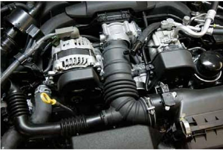
24. Next, we want to remove the air intake pipe in preparation for fitting the other parts of the turbo kit. Take your screwdrivers and loosen off the clamps on the inlet pipe at the throttle body and air box. Loosen off the clamp going to the sound box. Pull the smaller breather line hose off the inlet, then with that out, pull the inlet up and off the engine. You will not be using any part of it after this.
