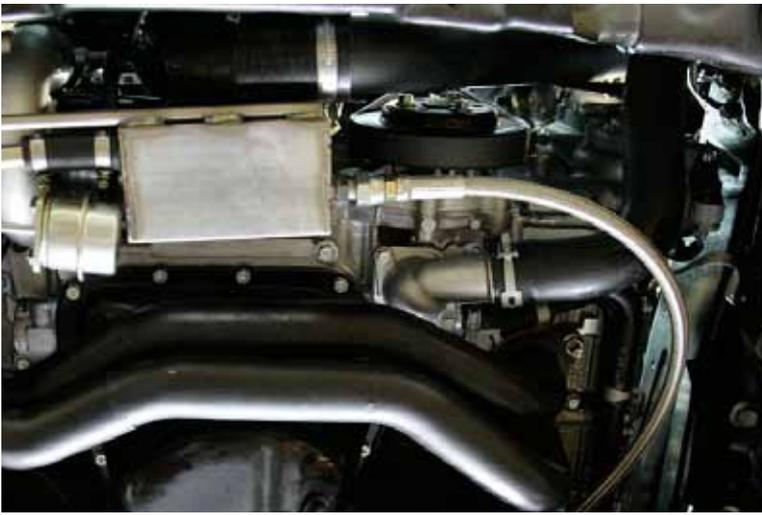
52. With the exhaust manifold fitted up to the car, and the turbo discharge pipe fitted up to the rest of the exhaust, you can now hook up the oil line from the pump to the oil reservoir tank.
