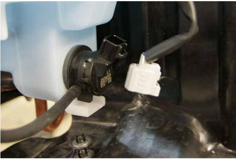
12. Lastly, unclip the wiring harness from the pump, and pull the water line off. Plug that off, and pull the water tank up and out of the car.
