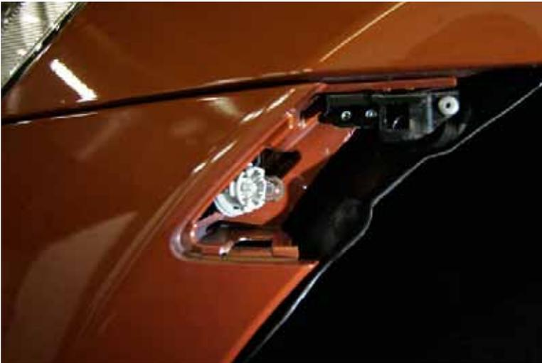
5. You will need to reach back behind there and unclip the light from the signal lamp housing. It's a push-in and twist type. With it removed, carefully pull the side marker housing out, exposing the pop-its inside that clip the bumper to the fender. Remove those pop-its.
