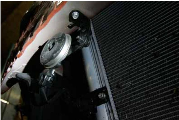
10. At the front of the radiator is a secondary horn. Unclip the wiring harness from it, and then unbolt it and it's bracket completely.
