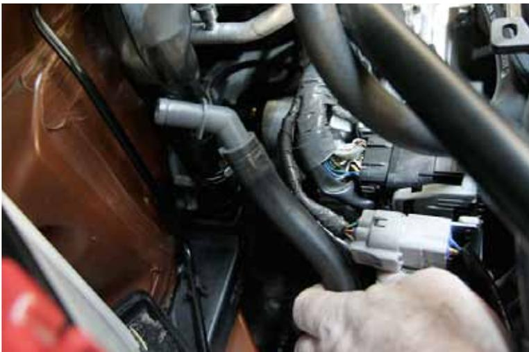
26. The sound tube from the back of the sound box goes into the firewall, in a recess that looks like it's part of the frame. It simply pulls out of a self-sealing socket inside there.
