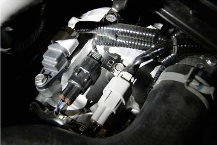
38. You may also want to loosen off this bracket that holds the secondary catalytic converter to the car. This is to give the system some wiggle room while removing and replacing the exhaust manifold.
