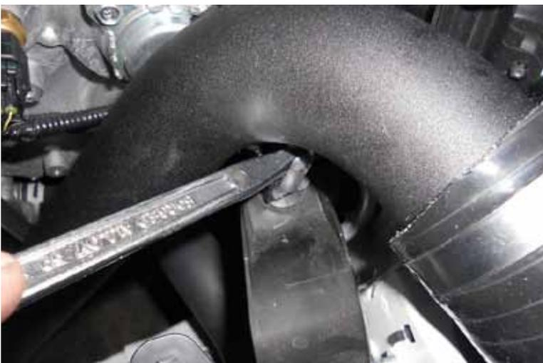
47. This bracket will attach to the air box mounting bracket at the front there. You need to use the metal spacer between the pipe bracket and the existing bracket for a nice, solid fit.
