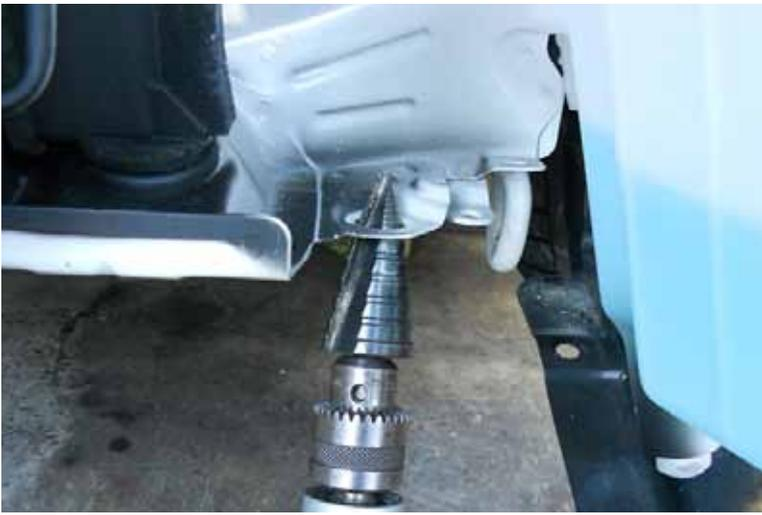
20. The windshield washer fluid tank mainly rests on a large hole at the bottom of the frame. What you will need to do is dremel it out to a larger size, this will enable you to shift the water tank down without removing the support entirely.
