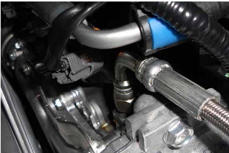
34. On the same side of the head as the oil pump, and near the front, there will be a large bolt at the top of the head. Remove it, and fit the oil fitting in its place. This is where the oil line will be fitted that goes to the turbo.
