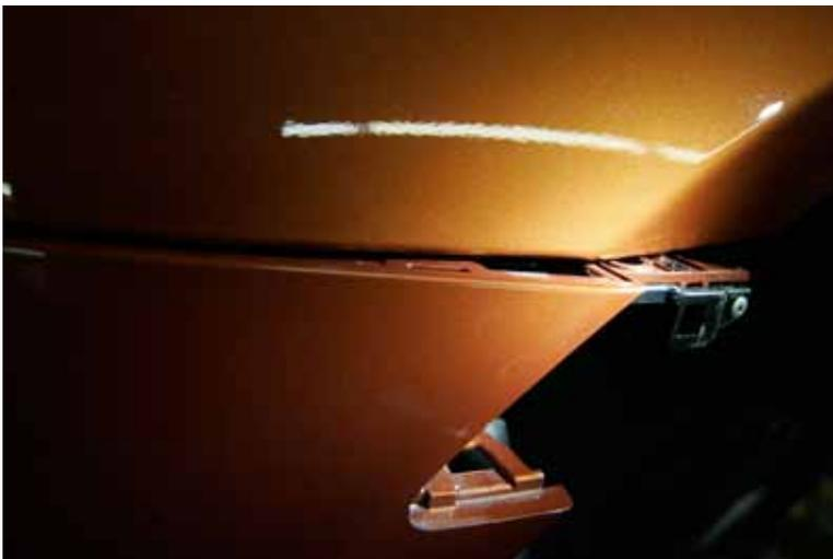
6. With all the pop-its removed, and all bolts un-bolted, all that is holding in the bumper is a series of clips along the top edge of the bumper where it meets the fender and the lights. For this step it's recommended to have two people to remove the bumper skin, as once it's off there is nothing holding it on. Carefully push in and up slightly to bring the bumper edge off the clips, and pull it out.
