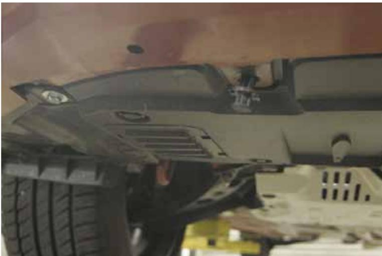
2. Along the front bottom edge of the bumper there is a combination of pop-its and regular bolts holding the bumper on. Remove the pop-its with a screwdriver, and then the bolts.
