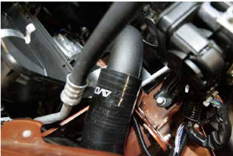
46. Finally, slide the metal pipe with the single bracket into the right side silicone hose (where the water tank is). The bracket needs to be at the silicone side.
