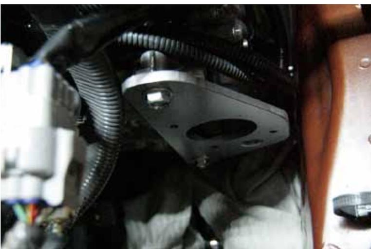
31. First, you need to remove the large plate from the supplied oil pump, and bolt it up lightly to get the placement figured out. Apply silicone sealant to the oil pump itself where it meets the plate, and fit the oil pump through the plate into the head, and get the rotation of the piece on the back of it right so that it slots into the head smoothly. Lightly bolt the oil pump to the plate - then remove the entire plate/pump from the head.
