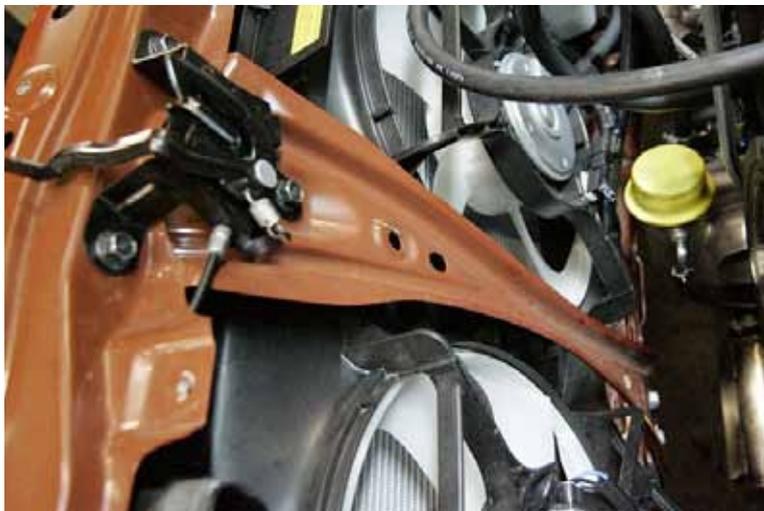
42. With the exhaust manifold out, now is a good time to tackle the this bracket. You need to unbolt it at the top and bottom, and take it off the car.
