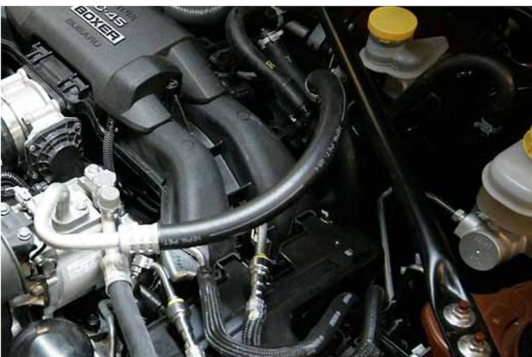
59. Now fit the air inlet pipe that will go from the airbox to the turbo. Fit it to the turbo first, and make sure it's clamped on tight. Run the breather line to the smaller fitting off the side, and clamp that in. Then prepare a clamp on the bigger fitting, this is where the BOV will fit into.
