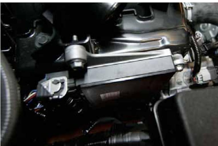
27. This is the computer running the injectors. For now, you will need to unplug the wiring harness, as you will be removing it and the black frame it's attached to so that you can get to some areas underneath. A small screwdriver is needed to slide in and unclip the wiring harness.
