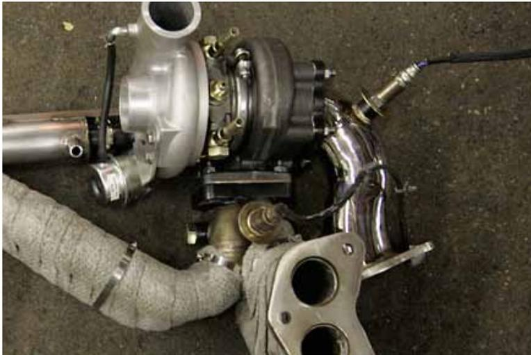
41. The pre-cat one goes onto the AVO exhaust manifold, and the post-cat sensor goes onto the turbo discharge pipe.
