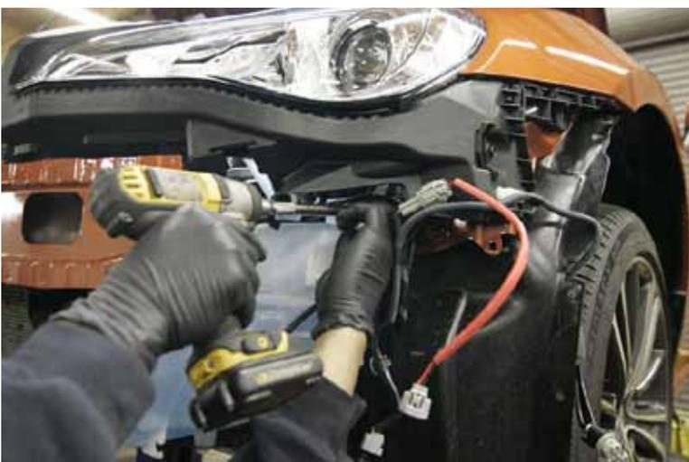
11. Finally, remove the water tank for now. It's advised to have a bucket to empty your windshield wiper fluid into until you finish. There is one bolt at the back to remove, and the top of water tank is held on by a screw-in type pop-it.
