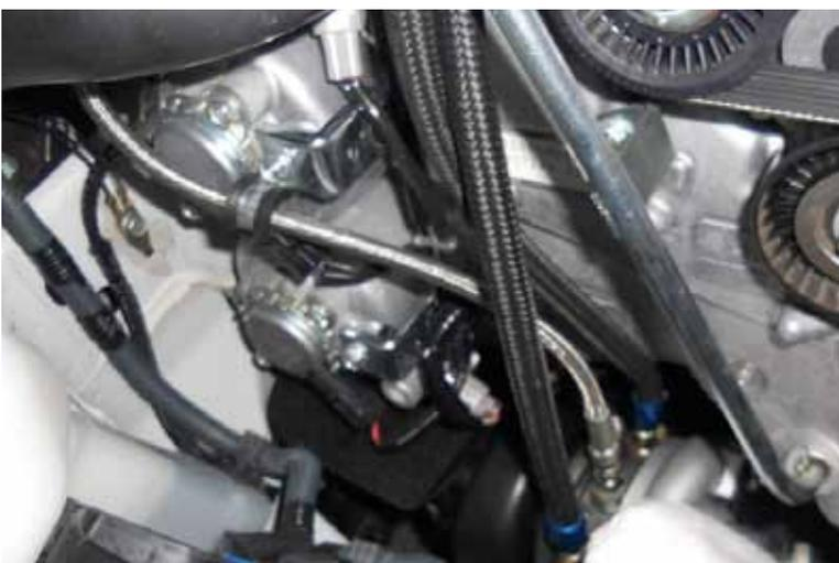
35. This oil line, once fitted, will come out the front side of the bracket once it's fitted back. However, wait till the turbocharger is fitted before fitting the oil line, as it's easier to fit the line to the turbo before the turbo goes on the car.
