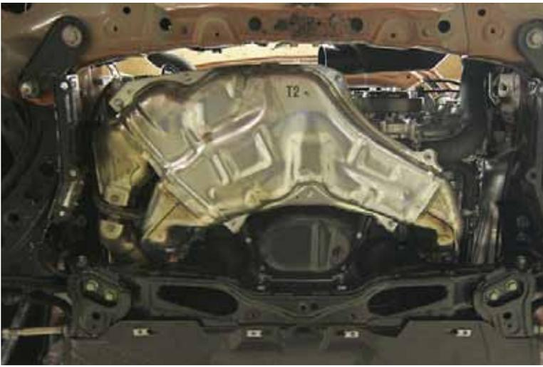
36. To fit the turbokit in place, you will need to completely remove the exhaust manifold. First unbolt the exhaust manifold from the engine crossover pipe.
