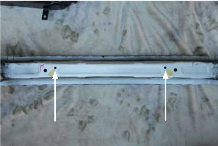
13. The easiest way to mount the FMIC is to remove the bumper beam off the car. At the back of the bumper beam is several holes. Find the two smaller holes towards the inside, these are the ones you will be mounting the FMIC to.
