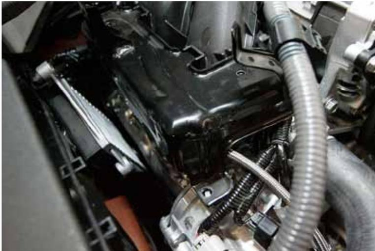
53. Screw the oil line off the turbo up to the oil fitting on the block. You can now replace the steel bracket that goes over that, and fit the fuel computer back as well, clipping the wiring harness back into it.
