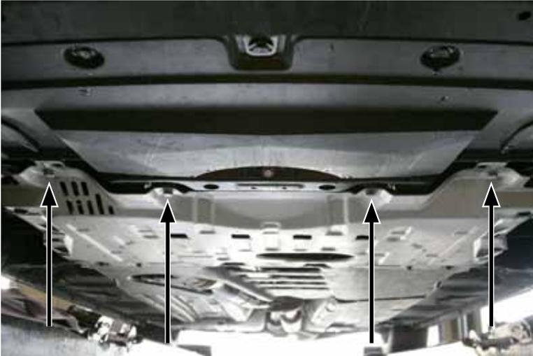
61. When fitting the front engine undertray back to the car, you should fit the supplied spacers at the front to ensure extra clearance for the exhaust manifold. They will be fitted to the 4 bolts at the front, as indicated.
