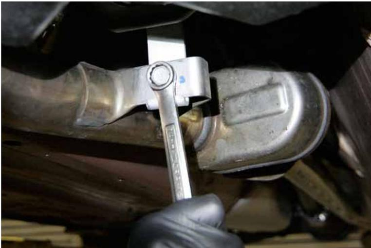
39. Using a socket wrench with a long extender, unbolte the exhaust manifold from the engine itself. You should be able to easily remove it completely at this point.
