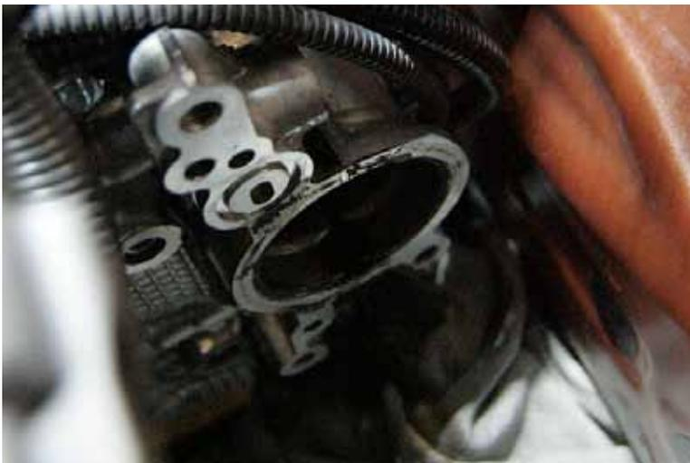
30. With the plate removed, you can see that there's a oil port and rotating clip assembly here. This is where the supplied oil pump will be fitted. These slots on the rotating assembly of the pump need to be fitted into their corresponding ridges inside the head.
