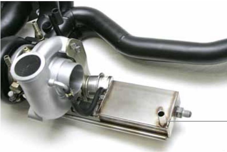
56. The metal fitting off the side of the oil reservoir tank is for a oil breather line, that will be tee'd between the standard breather line and the AVO inlet. It will need to be trimmed to fit, so that if you have an oil breather (oil/air separator) tank, the breather line will be long enough to go straight to that instead.
