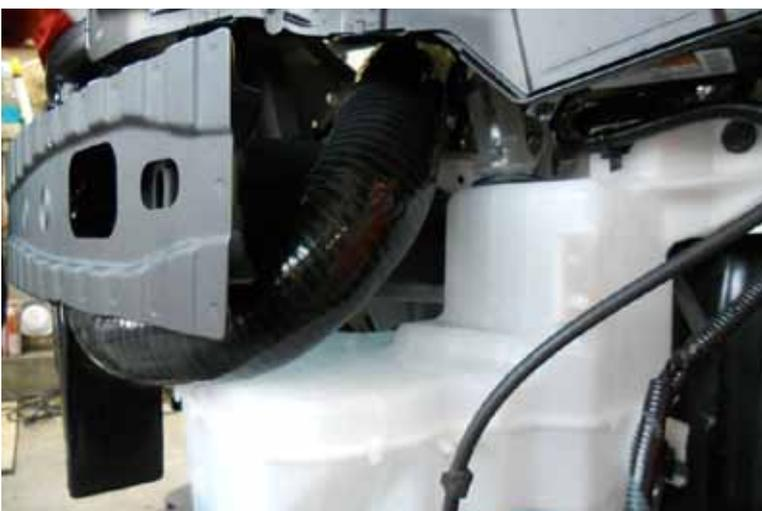
19. The right-side silicone piping will be passing through there up into the engine bay. To allow proper space to fit, you have a choice of slightly trimming the rear of the bumper beam in that location, or adjusting the location of the water tank a inch downwards. We will cover the water tank adjustment next.
