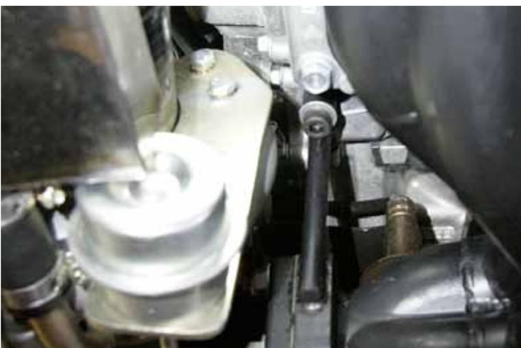
51. There is a bracket on the turbo flange of the exhaust manifold. This will bolt up to the engine here, using the supplied bolt.
