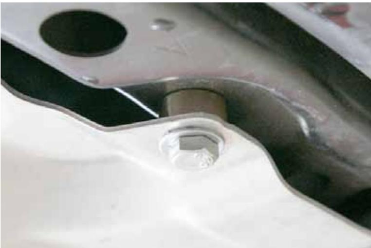
62. You will fit the spacer between the tray and the body of the car.
