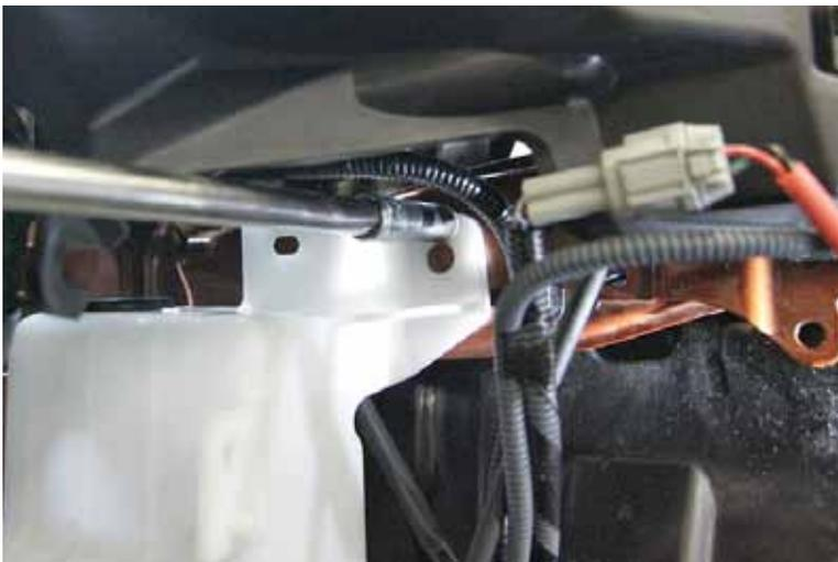
22. Next, slot the hold for the bracket at the back. You should be able to slide it into place at a lower point now. The water tank neck will stretch higher, so it can still bolt into place.
