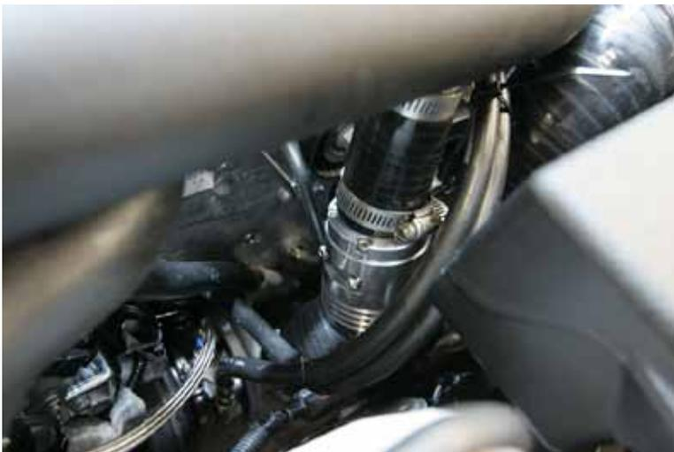
58. The BOV needs to be fitted to the underside of the intake pipe and clamped on. Then fit the intake pipe into the passenger side silicone hose (from the FMIC). Then fit the BOV discharge to the inlet pipe from the air box. Clamp all those together. Then fit the supplied small vacuum hose to the fitting on the BOV, and run it to the back of the engine where the vacuum line from the intake to the brake booster is.
