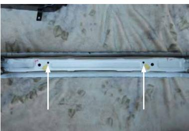
13. The easiest way to mount the FMIC is to remove the bumper beam off the car. At the back of the bumper beam is several holes. Find the two smaller holes towards the inside, these are the ones you will be mounting the FMIC to.
