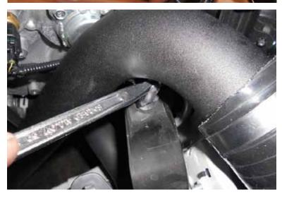
47. This bracket will attach to the air box mounting bracket at the front there. You need to use the metal spacer between the pipe bracket and the existing bracket for a nice, solid fit.
