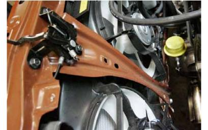
43. With it out of the car, you will need to modify it slightly at the bottom. As there will be silicone hosing resting against it once everything is installed, we recommend flattening down the outer edges so they don't cut into the silicone pipes. Then bolt it back in with the supplied rounded head bolts used at the bottom.
