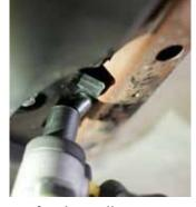
3. At the bottom of the tire fenderwall area, there is another pop-it as well. Then the fender liner is held in place with a series of smaller pop-its, you will need to "unscrew" these with a plus-head screwdriver.
