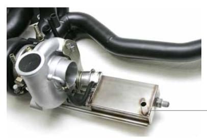
56. The metal fitting off the side of the oil reservoir tank is for a oil breather line, that will be tee'd between the standard breather line and the AVO inlet. It will need to be trimmed to fit, so that if you have an oil breather (oil/air separator) tank, the breather line will be long
