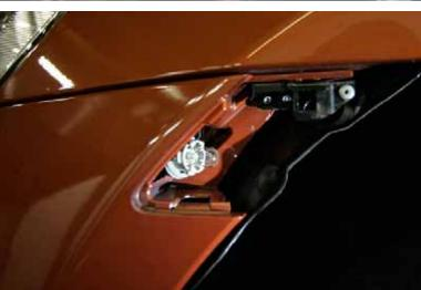
5. You will need to reach back behind there and unclip the light from the signal lamp housing. It's a push-in and twist type. With it removed, carefully pull the side marker housing out, exposing the pop-its inside that clip the bumper to the fender. Remove those pop-its.
