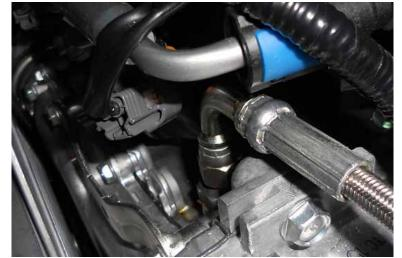
34. On the same side of the head as the oil pump, and near the front, there will be a large bolt at the top of the head. Remove it, and fit the oil fitting in it's place. This is where the oil line will be fitted that goes to the turbo.
