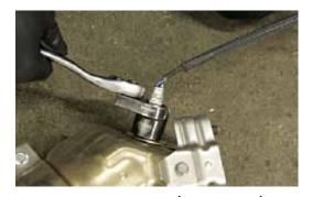
41. The pre-cat one goes onto the AVO exhaust manfold, and the post-cat sensor goes onto the turbo discharge pipe.
