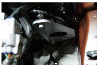
31. First, you need to remove the large plate from the supplied oil pump, and bolt it up lightly to get the placement figured out. Apply silicone sealant to the oil pump itself where it meets the plate, and fit the oil pump through the plate into the head, and get the rotation of the piece on the back of it right so that it slots into the head smoothly. Lightly bolt the oil pump to the plate - then
