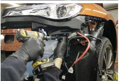
11. Finally, remove the water tank for now. It's advised to have a bucket to empty your windshield wiper fluid into until you finish. There is one bolt at the back to remove, and the top
