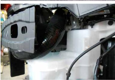
19. The right-side silicone piping will be passing through there up into the engine bay. To allow proper space to fit, you have a choice of slightly trimming the rear of the bumper beam in that location, or adjusting the location of the water tank a inch downwards. We will cover the water tank adjustment next.
