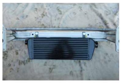
16. Screw the FMIC down to the bumper beam. Make sure it is snug against the bottom of the inner bumper beam.
