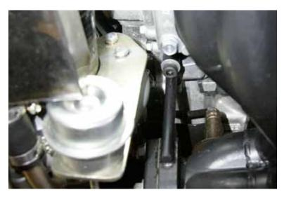
51. There is a bracket on the turbo flange of the exhaust manifold. This will bolt up to the engine here, using the supplied bolt.
