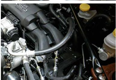
59. Now fit the air inlet pipe that will go from the airbox to the turbo. Fit it to the turbo first, and make sure it's clamped on tight. Run the breather line to the smaller fitting off the side, and clamp that in. Then prepare a clamp on the bigger fitting, this is where the BOV will fit into.
