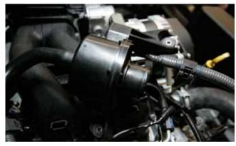
26. The sound tube from the back of the sound box goes into the firewall, in a recess that looks like it's part of the frame. It simply pulls out of a self-sealing socket inside there.
